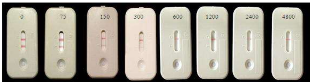
Figure 1. A semi-quantitative competitive lateral flow assay with powdery mildew conidial numbers tested between 0 – 4800
