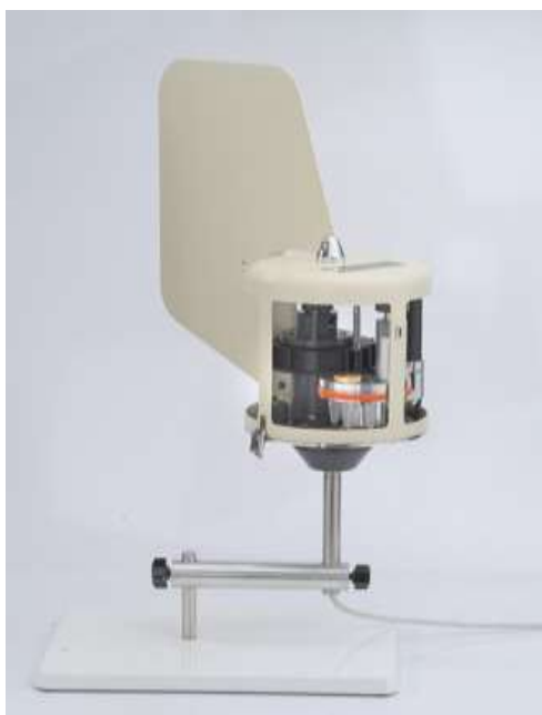
Figure 2. Burkard multi-vial 8 day air cyclone sampler
